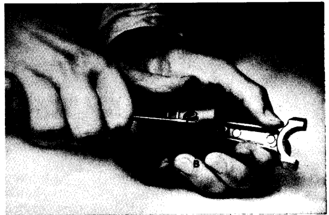
Figure 71. Disassembly of Rod and Piston.
