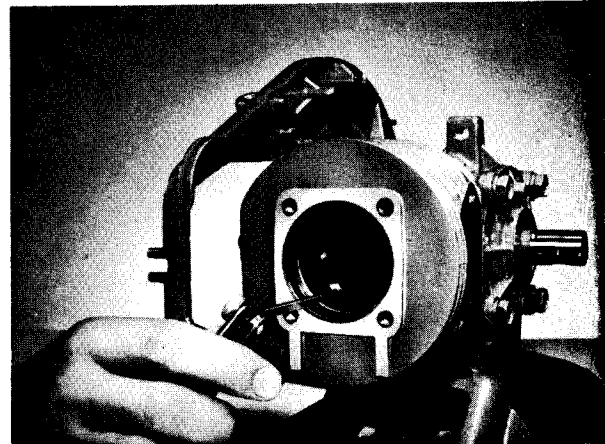
Figure 74. Piston Ring Gap Test.
